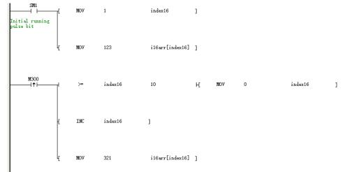
2. Start assigning 123 to i16arr[1], after which each trigger of M300 will assign 321 to each of the following array elements; After startup, the result is as shown in the following figure:
