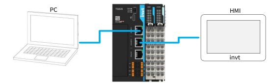
In the example figure, Ethernet 1 is connected to Auto Station Pro in the upper computer to upload/download programs, and Ethernet 2 is connected to HMI for data display.
