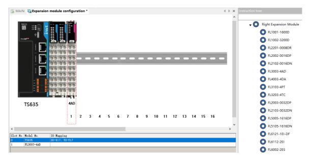
Step 2 When the local analog input expansion module is connected to the main module, double-click the module to pop up the module configuration interface, and configure the channel setting, conversion mode and IO mapping according to the actual demand.
