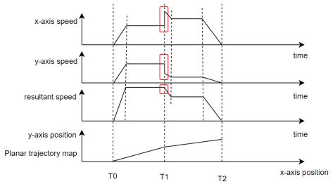
Note: At time T1, the linear interpolation was interrupted, and it can be seen that there was no jump in the "resultant speed" at T1;At T1, both the "x-axis speed" and "y-axis speed" experienced a jump. If a single axis needs to undergo reverse motion,Then the speed of the axis will undergo a reverse jump from positive to negative.
