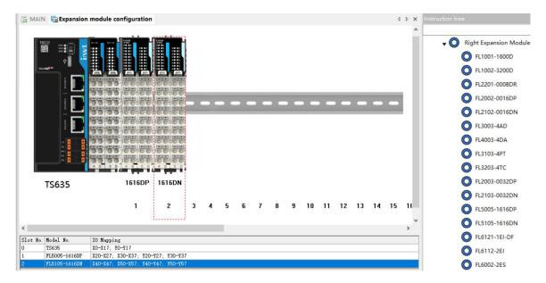
Step 2 When the hybrid expansion module is connected to the main module, double-click the module to pop up the module configuration interface. In the "Parameter Setting" interface, configure the "Filter parameter 1," "Filter parameter 2," and "Stop output mode" according to actual needs. In the "IO Mapping" interface, configure the "IO Mapping."
