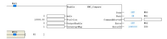
Step 4 When the encoder position value is equal to the comparison value, the interrupt service function INT\_1 is triggered to light up Y0.
