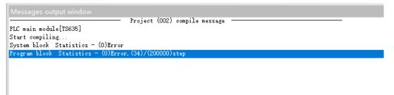
Step 2 After successful compilation, you can click the Download button in to download. When downloading the program, PLC must stop. If PLC is running, the system will prompt with a dialog box, as shown in Figure 2-10.
