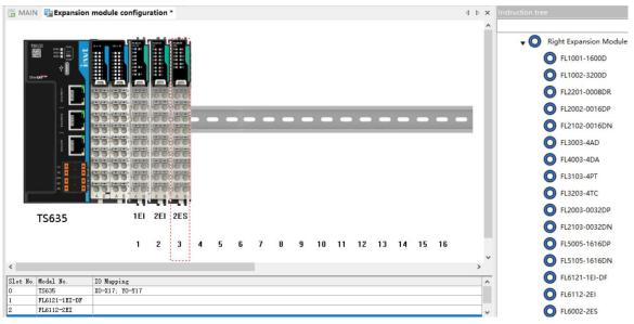
Step 2 When the counter expansion modules are connected to the main module, double-click the module to pop up the module configuration interface, and configure the parameters and IO mapping according to the actual demand.
