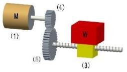
Where, (1) is a servo motor, (3) is a workpiece, (4) is the denominator of gear ratio, and (5) is the numerator of gear ratio.
