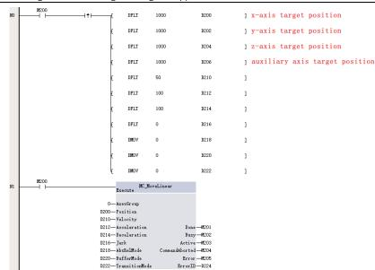
**Note:** The parameter "Position" of MC\_MoveLinear is an array of length 4 with members of REAL type. The data length of D200 – D201 is also of REAL type, so you only need to assign the X-axis target value of 1000 to D200. Similarly, the Y-axis target value is assigned to D202, the Z-axis target value is assigned to D204, and the auxiliary axis target value is assigned to D206. At the same time, the next parameter "Velocity" should be allocated from the memory segment after D208.
