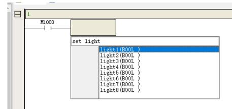
Elements are used directly for custom variables, so in actual use, the interface displays the element name.
