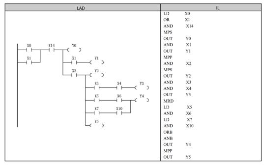
Figure 5-3 Conversion of Ladder Diagram into Instruction List
