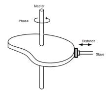
The electronic cam just imitates this structure, where an axis is chosen as the master axis with the other axis as the slave axis, and both of them move synchronously according to the set cam curve.
