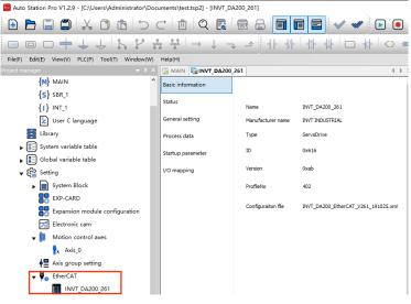
Step 6 Choose "AXIS\_0" and the output device "INVT\_DA200\_171" to associate the axis AXIS\_0 with the INVT\_DA200\_171 servo driver
