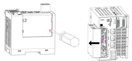
Step 4 Slide the expansion card into the guide slot horizontally, and then press the snap positions on the upper and lower sides of the expansion card hard until the expansion card is snapped tightly (there is obvious snap sound after it is installed in place).
