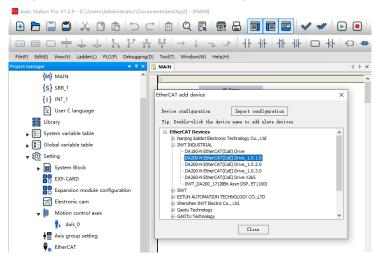
Step 5 The DA200 servo driver slave is created, and the EtherCAT add device interface is closed
