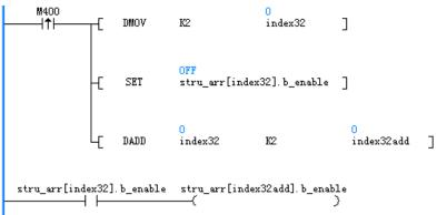
2. After M400 is triggered, set stru\_arr[2].b\_enable, and control stru\_arr[4].b\_enable, as shown below:
