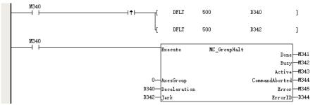
**Note:** MC\_GroupHalt can be pulled up again to interrupt itself and will execute according to the latest module parameters. When multiple MC\_GroupHalt function blocks run with the same axis, the latter function block will interrupt the previous module and the previous one will be displayed as being interrupted.
