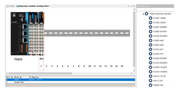
Step 2 When the local analog output expansion module is connected to the main module, double-click the module to pop up the module configuration interface, and configure the channel setting, conversion mode and IO mapping according to the actual demand.
