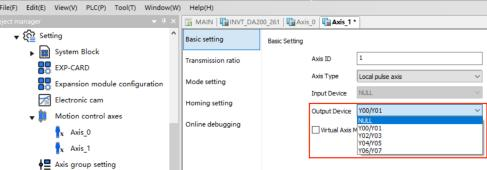
Step 4 The configuration of local pulse axis and fieldbus servo axis is completed.
