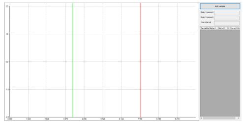
Step 3 Click "Add Variables" in Figure 2-14, and choose the main task from the associated tasks in the "Variable setting" pop-up window. Set variables D0, R0 and VAR\_01 to be captured, and then click "OK" to save the variable settings.
