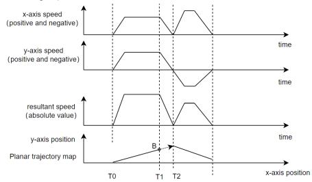
Note: At time T1, the function block needs to be pulled up again to interrupt itself, which is point B, and the y-axis needs to run in the opposite direction because the "interrupt deceleration to zero" is selected. Here, the y-axis and x-axis first decelerate to zero together (as shown by the dashed arrow between T1 and T2), then accelerate from T2 to the new target position, so that there is no speed jump during the speed change process.
