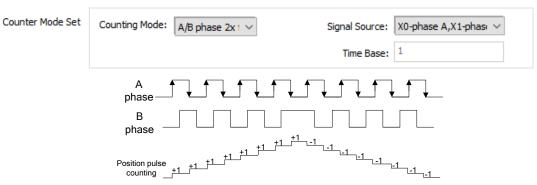
In the A/B phase 4 frequency doubling mode, the rising/falling edge of the A-phase pulse and B-phase pulse is counted, as shown in the following figure.
