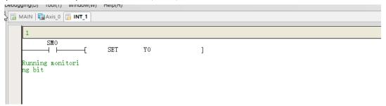
Step 3 Configure the corresponding Interrupt number for "Interrupt" in the instruction ENC\_Compare and start IE.
