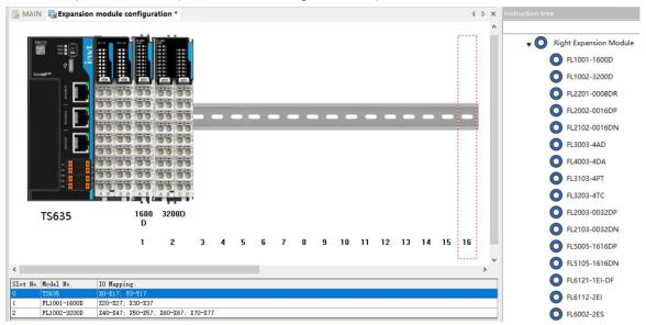
Step 2 When the local digital input expansion module is connected to the main module, double-click the module to pop up the module configuration interface, where you can configure the filter parameters and IO mapping according to the actual demand. If the mapping variable is not manually configured by the user, the input X port number on the expansion module is followed by the X port number on the main module or the previous digital input module, and is numbered in turn.
