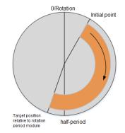
Reverse: First, the target displacement is modulated against the rotation cycle, and then the axis runs counterclockwise from the starting position of the axis to the target position.
