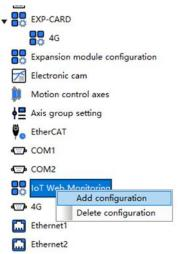
Step 3 Double-click the "Web monitoring configuration" button to pop up the web monitor configuration bar.
