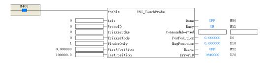
The parameter "ProbeID" indicates the probe number used by the encoder axis as follows:
