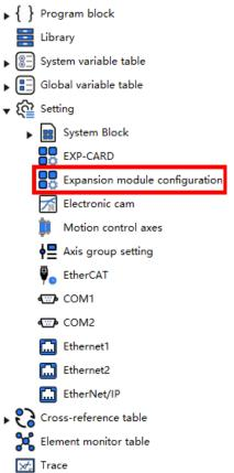
2. Switch to the expansion module configuration interface, double-click the module on the right side to automatically expand it on the expansion rack, or drag it to the expansion rack with the left mouse button.
