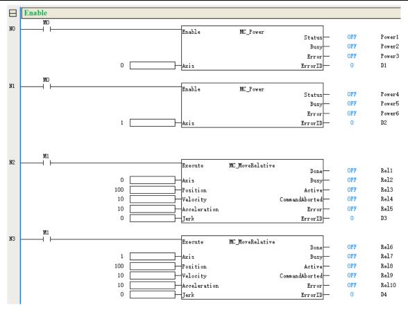
Step 2 Double-click to select Axis 0, and click online debugging to observe the enable status and communication status of the axis
